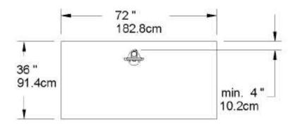
The minimum space requirements for High Security Bike Pumps are meant to allow a cyclist and their bike access to the pump.
