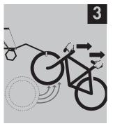
Grasp bike by seat and handlebars and pull backwards to initiate lifting mechanism.
