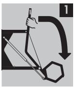
Pull down lifting arm into fully lowered position.
