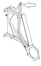
The Tip-Up arrives fully assembled aside from the wheel hook. This will need to be inserted and secured to the end of the lifting arm.
